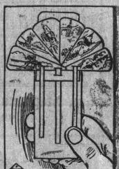
tangular box. In the back of the back is a slide which is connected to each card. Normally the entire box pre-Guides are attached to each earn and also to the slide to limit the withdraw all movement and to present the cards in a neat agrangement. A series of scenes in rotation or a number of local views add considerably to the attractiveness of the card. The latter is mailed in the usual way, the name and residence of the addressee being placed on the reverse side.
