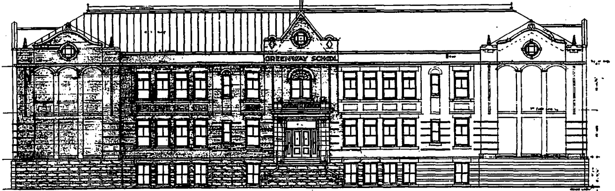
Front elevation, Greenway School, Winnipeg, now under course of construction. The walls are being built of buff brick and Tyndall stone, a combination of materials used in the exterior of all Winnipeg schools.
