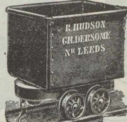
70—R.H.'s Patent Steel Mining Wagon
