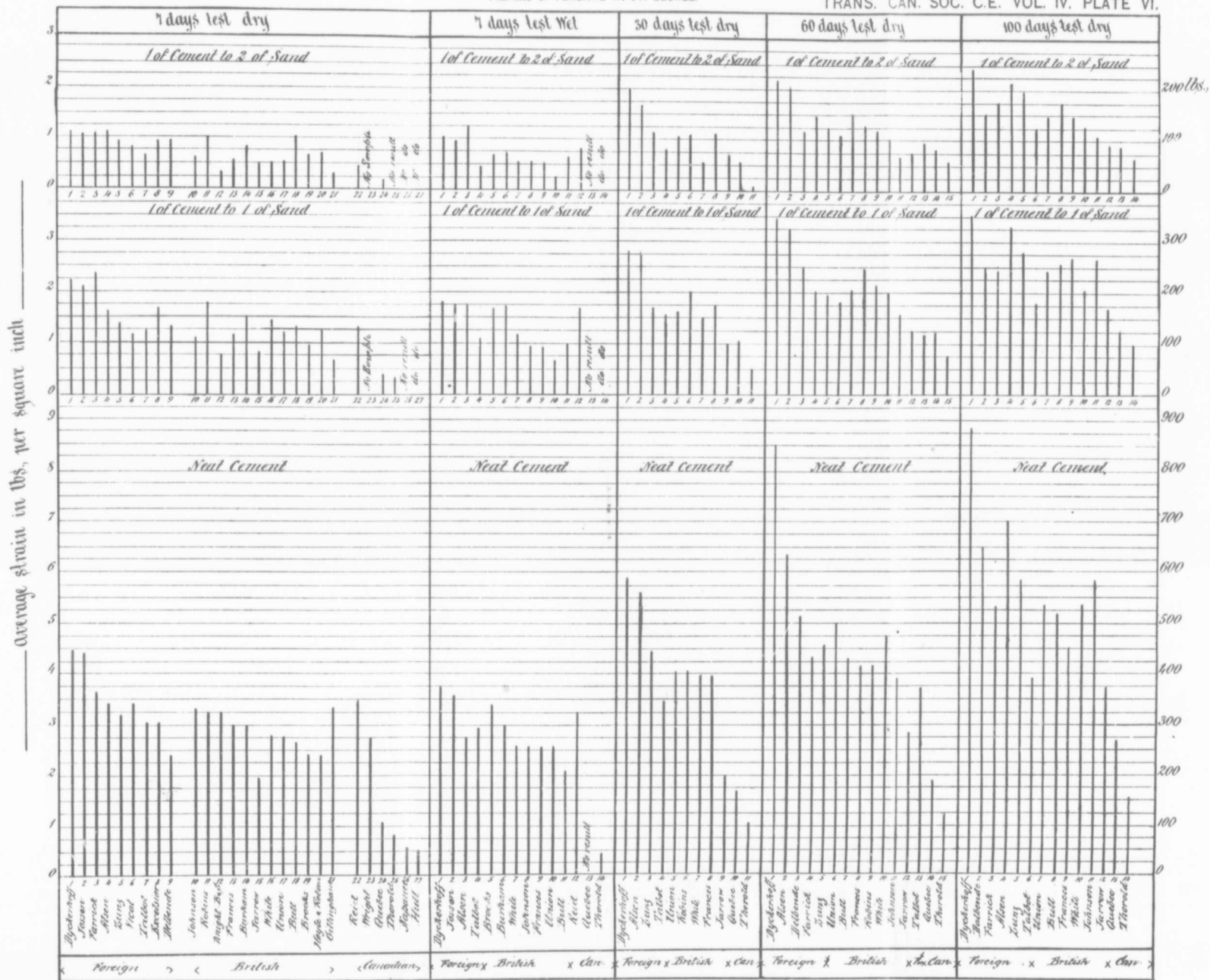
DIAGRAM SHOWING RESULTS OF TESTS MADE WITH VARIOUS CEMENTS, TO ACCOMPANY DISCUSSION ON MR. BUTLER'S PAPER ON NAPANEE CEMENT.
