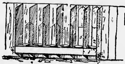
Partitions Built on Inside of Paddock Fence.
