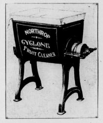
is built entirely of metal and is the most efficient, durable and yet simple fruit cleaner ever invented. It will clean over 1,000 lbs. of currants per hour and leave the fruit with the natural bloom revived, the skins uninjured and apparently of a higher grade than before, ready for immediate packing or using in any form required. Sole owners and patentees for Canada,
