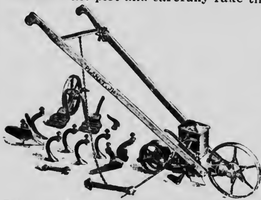
Fig. 12.—Garden Hand Drill with Attachment for Sowing, Hoeing, Cultivating and Hilling.
