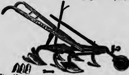
Fig. 13.—Horse Cultivator for use in Gardens where Vegetables are planted in long rows.
