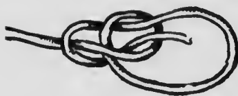
Bowline: a noose that neither jams nor slips.
