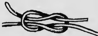
Reef knot or square knot: never slips or jams; easily loosened.
