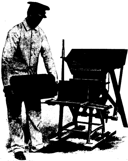
The "IDEAL" Concrete Block Machine. The original Face-down, Horizontal-core Block Machine, and the only one of its kind that can be legally made and sold in Canada.
