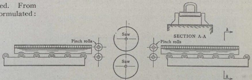
Sectional View of Machine for Carrying Out Deseaming Operation.
