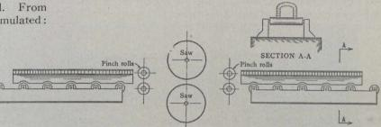
Sectional View of Machine for Carrying Out Deseaming Operation.
