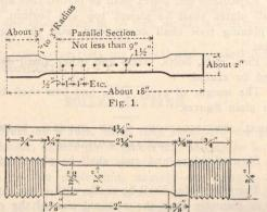
9. Material which is to be used without annealing or further treatment shall be tested in the condition in which it comes from the rolls. When material is to be annealed or otherwise treated before use, the specimen representing such material shall be similarly treated before testing.
