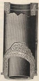
Concrete Tile and Mould.
