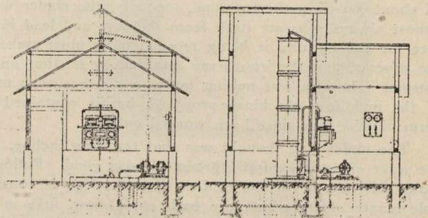
Fig. 2.—Water Sterilising plant for Operation on 110-220 volt Direct Current Circuits. Output 2,200 Gallons per hour.
