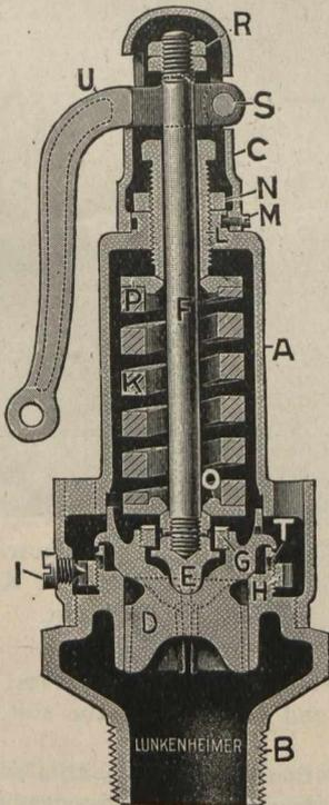
bronze composition, insuring great durability; are very simple in construction, and are warranted to be reliable, accurate and positive in operation. They have full relieving capacity, are very sensitive to excessive pressure, and admit of being finely adjusted. The valves are provided with
