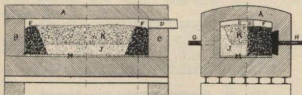
Fig. 31.—Johnson's Electric Zinc Furnace.
