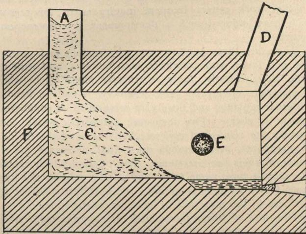
Fig. 32.—de Laval's Electric Zinc Furnace.
