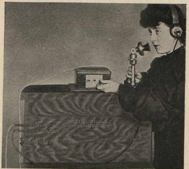
Fig. 4.—One of the Sending Stations Showing Head Receiver Used by Soloist to Assist Her in Keeping Time With Accompaniment.
