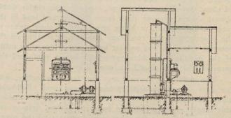
Fig. 2.—Water Sterlising plant for Operation on 110-220 volt Direct Current Circuits. Output 2,200 Gallons per hour.
