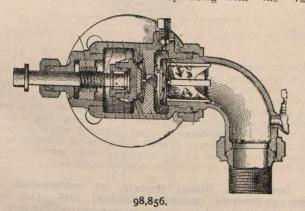
seat, and a central tongue portion fitting closely within the aperture of the valve seat. A check valve is arranged in said casing below the stop valve having on its top side a central boss and raised an-nular rim at the periphery projecting beyond said central boss, a spider having a central portion adapted to stop
