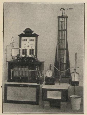
Fig. 1.—Ozone Sterilisation Apparatus for Bacteriological Research Work.
