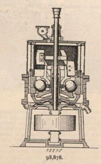
supported in said casing to the outer side thereof and be-tween said screen and the said central shaft are arranged a plurality of rotatable wings having plates obliquely arranged thereon and forming the means for elevating the ground substance and bringing the same into contact with the said screen thus allowing all coarser particles to drop back freely to the grinding mechanism.
