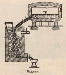
metallic vapors—for instance, such as molten silicates (in-cluding slag, scoria, cinders and the like) or a molten metal, as iron—the heat carrier being heated above its melt-ing point up to incandescence.
