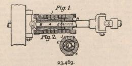
circling parts of the sleeves B, H by the spring J is that upon the spring J being subjected to torque, and becoming reduced in diameter, its ends engage the parts of the sleeves after the manner of a coil clutch, and thus take a proportion of the driving effort, so relieving the anchors of the spring.
