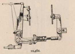
oted to an adjusting device, which is pivoted at its other end to a lever connected with one of the brake beams, being a third brake lever connected to the main brake lever by a pivot pin.
