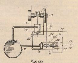
In operating a gas-engine where the combustion is accomplished by means of an electric sparking apparatus it
