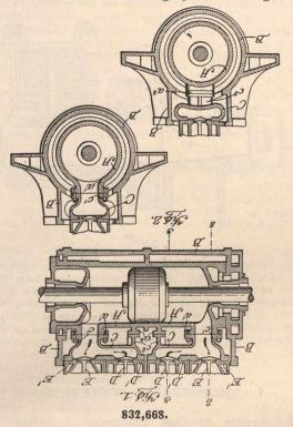
a flanged junction, a water-jacket surrounding the working cylinder a d extending above the flanged junction and the rib, and a valve-chest provided with a rib and a flanged junction supported respectively on the rib and the flanged junction of the working cylinder in such a manner as to permit relative expansion movement between the chest and the cylinder and located within but spaced from the walls of the water-jacket.
