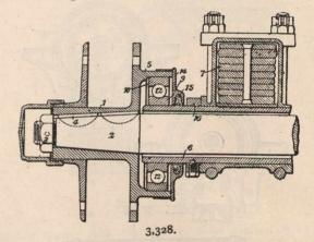
packing 15 being provided in a recess in the surface adjacent to the said tube. Lateral movement along the tube 6 of the parts constituting the ball bearing may be limited by a removable ring or a collar 16 on the tube; the caps or covers 14 of the two bearings of an axle can be arranged to bear against rings or collars 16 on each end of the tube, and thus to limit lateral movement in either direction.
