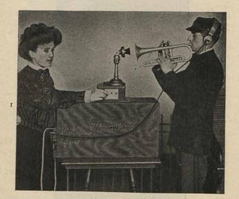
Fig. 3.—Sending Station Apparatus, with Cornetist Playing Directly in Front of Transmitter.
