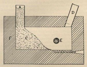
Fig. 32.-de Laval's Electric Zinc Furnace,
