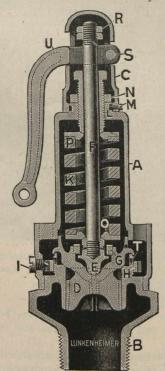
bronze composition, insuring great durability; are very simple in construction, and are warranted to be reliable, accurate and positive in operation. They have full relieving capacity, are very sensitive to excessive pressure, and admit of being finely adjusted. The valves are provided with lock-key attachment, to guard against their being tampered with, and adjustments of pop lid and pressure can be made from the outside of the valve without taking it apart.
