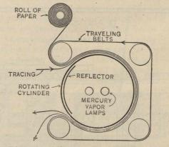
Fig. 1.-Diagram of Electric Blue-Printing Machine.
