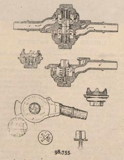
The spring-held valves are held from their seats by their inner faces abutting each other when the interlocking portions are secured together and have a small orifice through the valve portion allowing the air to escape grad-ually instead of rushing out of the larger opening on the disconnection of members.
