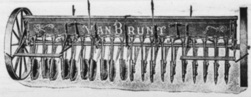
Made in 12, 14, 16, 18, 20, 22 and 24 Single, Double Disk and Shoe Interchangeable
