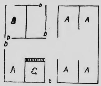
Figure 94.—Ground floor plan of barn shown in figure 93. A good farm barn. A—open stalls; 11—box stalls; G—grain.
