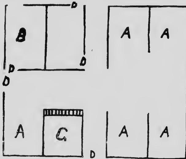
**Figure 94.**—Ground floor plan of barn shown in figure 93. A good farm barn. A—open stalls; I—box stalls; G—grain.
