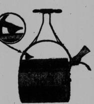
This roller can be made as heavy or as light as desired by simply putting in the right amount of water or sand. The advantage of this is obvious, for you are not handling any extra weight and for storing away it can be emptied entirely.
