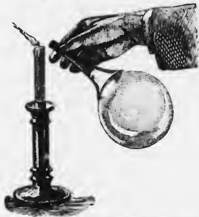
FIG. 1. THE CONTRACTING BUBBLE BLOWS THE FLAME.
