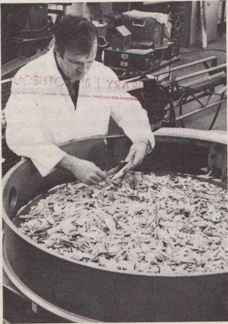
*A researcher examines residue wood chips such as are produced in most mills. These residues could be used in biomass gasification to produce fuel such as methane.*
