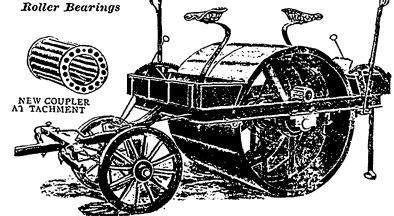
With Roller Bearings and New Patent Coupler Attachment, either 21/2, 31/2, 41/2 or 51/2 tons. All one size frame, drum, and width of tread and can be extra weighed 2 tons each. Address for Catalogue
