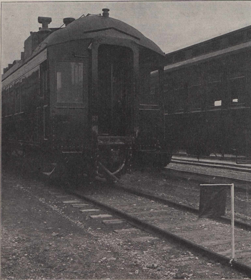
Fig. 1.—Blue Flag on Rail in Front of Passenger Car. (Car not undergoing Repairs.)
