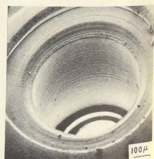
These micrographs show meter pivots from Bach-Simpson Ltd. of London, Ontario. Meter movements using these pivots showed a tendency to stick. Corrosion on the steel point (upper left) was found to be a contributing factor. The ruby insert bearing in the threaded brass rod (lower micrographs) shows no wear marks or irregularities.
