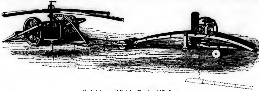
Fowler's Improved Draining Plough and Windlass.
