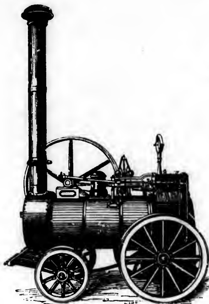
Burrell's Six-horse Portable Steam Engine.
