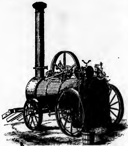
Clayton and Shuttleworth's Six Horse-power Portable Steam-engine.
