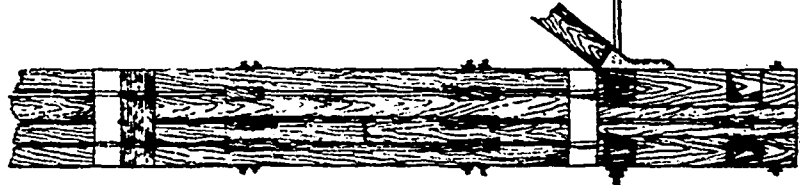
DETAIL OF BOTTOM CHORD
