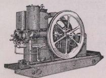
Skidded Evaporator Tank Engine 5 and 8 H.P.
