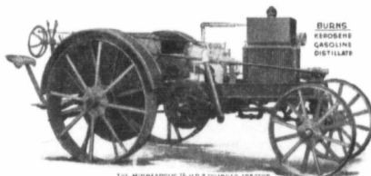
THE MINNEAPOLIS 20 H.P. 4-CYLINDER TRACTOR ALL GEARS ENCLOSED AND RUN IN OIL
