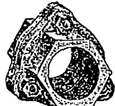
Improved Bolt Union for Steam Tubes.
