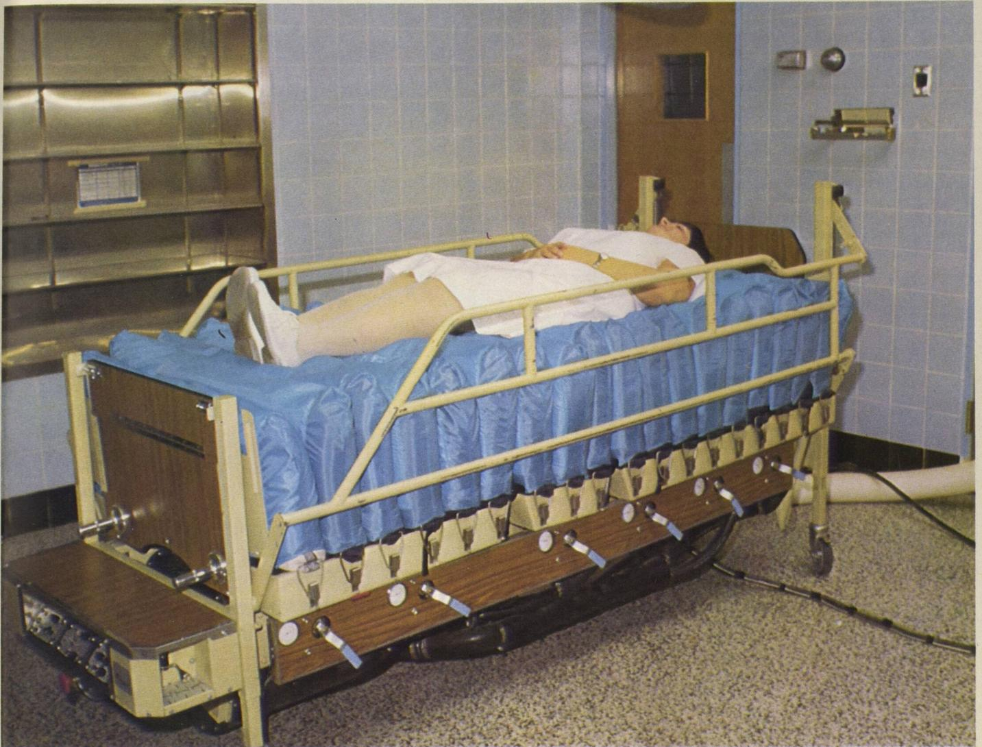
Using the same principle as an air cushion vehicle, this experimental hospital air bed supports a patient on a film of air. The Engine Laboratory built the bed for clinical evaluations and the study of new techniques for the treatment of burns. (Photo: Division of Mechanical Engineering)
