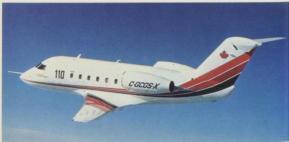
Canadair's Challenger, a new executive jet, outperforms all the competitors in its class while using less fuel. NAE investigated its design by studying a model in the trisonic, 1.5 m wind tunnel operated by the High Speed Aerodynamics Laboratory. The aircraft's windshields, tail assembly and engine nacelles were tested by the Structures and Materials Laboratory for their ability to withstand collision with birds while in flight. (Photo: Canadair Ltd.)
