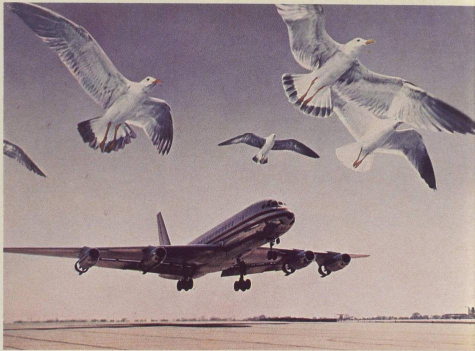
NAE has investigated several methods of discouraging birds from airfields to prevent collisions with aircraft. But, since collisions cannot be avoided altogether, NAE operates a facility to assist manufacturers in determining whether key structures such as windshields, tail assemblies and engine nacelles can safely withstand collision. (Photo: National Aeronautical Establishment)
