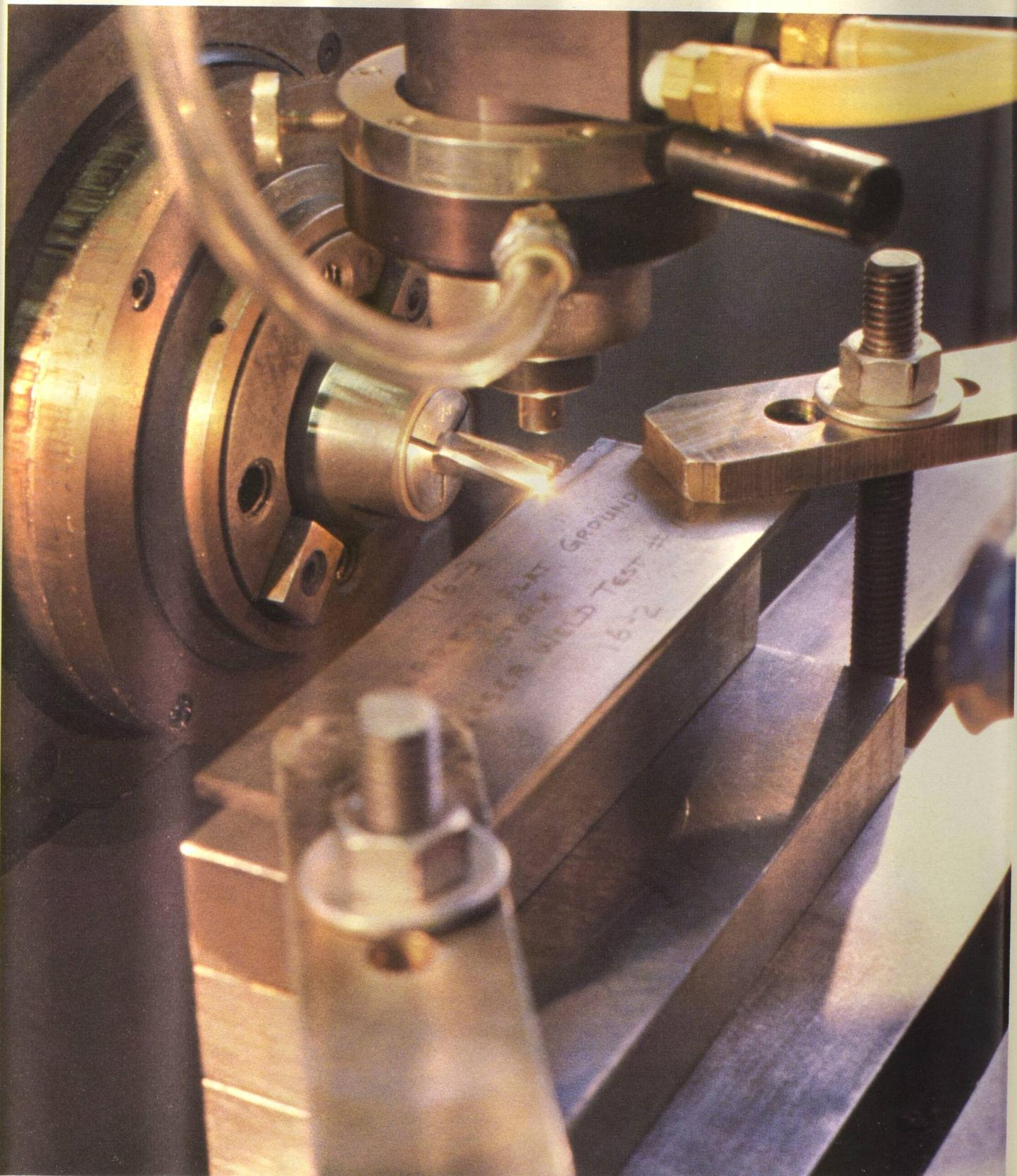
The Manufacturing Technology Centre is experimenting with the use of a laser beam for localized heating of a hardened workpiece immediately before machining. This allows the use of conventional machine tools such as lathes to produce parts from materials that are normally too hard to machine.
