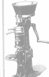
Stand, Square Gear, One-piece Skimmer, and all other parts, are made strong enough to last fifty years? There is no wobbling of the Bowl, because it is supported at both ends (MAGNET patent). Skims as perfectly in twenty years as at first. Separates foreign matter from milk and cream. Skimming capacity increased for a few dollars at a time by changing the Bowl and Skimmer only.
