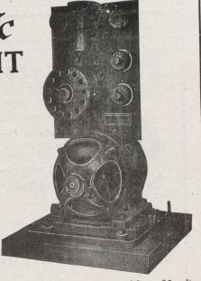
Northern Electric S-8 Belt-driven, 32 volt Electric Plant
