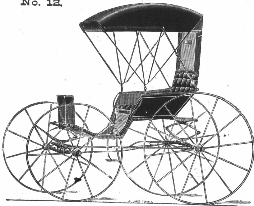
END SPRING PHÆTON on McLaughlin Patent End Spring Gear. McLAUGHLIN PATENT LOCK LEVER TOP.
