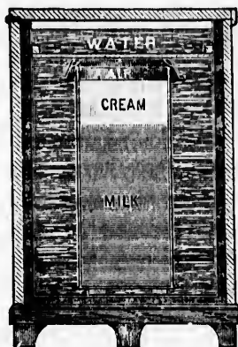
FIG. 104.—SECTIONAL VIEW OF COOLEY CAN AND CREAMERY.
