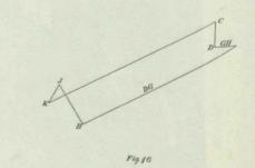
and the length of the line GH gives the magnitude Combine these four vector diagrams in one (fig the tension in the member GH.
