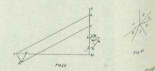
and the set of forces becomes GF, GH and R2 (Result ant of FN and NH) S Draw the vector diagram GF, and GH and R2, fig. 19 ant of FN and NH) fig. 12.
