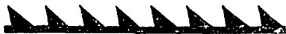
Garnett Wire. This Wire is used for covering iron rollers, breasts of woolen cards, lickers in of cotton cards, comber doffers, etc
