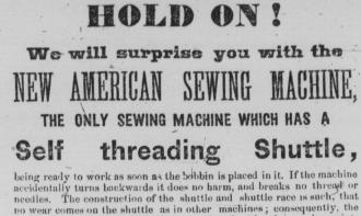
no wear comes on the shuttle as in other machines; consequently, the shuttle does not wear sharp and cut the thread. Also the wearing points of the machine are adjusted on steel centres, thereby avoiding friction, and adding greatly to its durability
