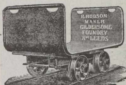
76—Hand Trolley, made to carry any weight or to suit any rail gauge.
