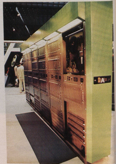
Northern Telecom's DMS-100 (digital multiplex system) switching machine at Telecom 83. It has a capacity of up to 100 000 lines and can relate to Integrated Business Networks, integrated voice and data terminals, Autovon military network, Maintenance and Administration Positions (MAP) and Traffic Operator Position Systems (TOPS).
