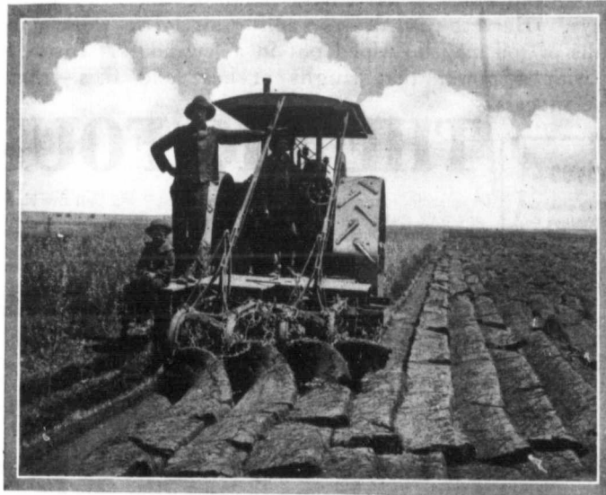
An I H C Tractor Pulling a 4-Bottom John Deere Engine Gang
