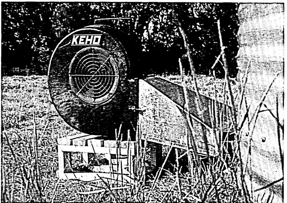
*The KEHO Natural Air Drying/Aeration System with 3 H.P. Hi-Flow Blower dries 3000 bu. of 18-per-cent moisture wheat.*
