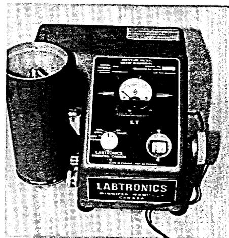
*Labtronics' Model 919 grain moisture meter with patented "cone" cell.*
