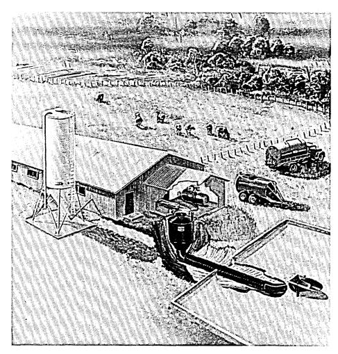
The Evacuair from Équipement Agricole Côté Inc. is an underground manure removal system.
