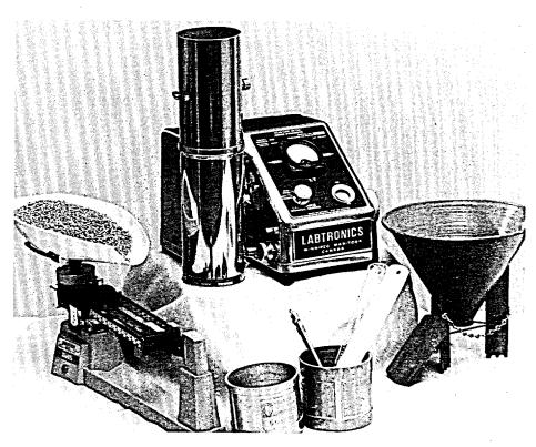
Labtronics offers the Model 919 moisture meter, scale/balance, ½ L measure, pint measure, thermometer, rapeseed kit and cox funnel, all required for moisture and weight determination.
