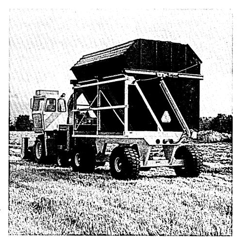
TY-CROP's 12-ft. Model TY-DUMP self-unloading forage wagon offers heavy-duty construction and trouble-free operation and is ideal for all silage crops, as well as the harvesting of vegetable crops.
