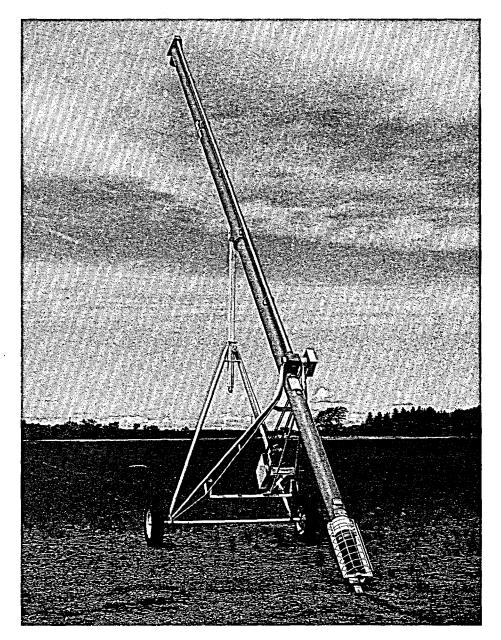
The Farm King Allied Portable Grain Auger features a telescoping lift system for greater height and reach.
