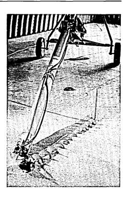
Wheatheart's Hydrostatic Binsweep features variable speed and pressure relief all in one valve for the utmost in operator safety.
