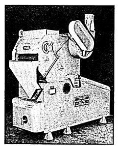
Simon-Day manufactures the Carter Screen Machine, a total seed and grain cleaning machine that combines the features of a scalperator and a gyratory screen cleaner.
