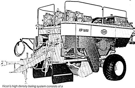
Vicon's high density baling system consists of a hydraulic high density baler for the harvest and a loader with three-bale gripper and trailers to transport the bales.
