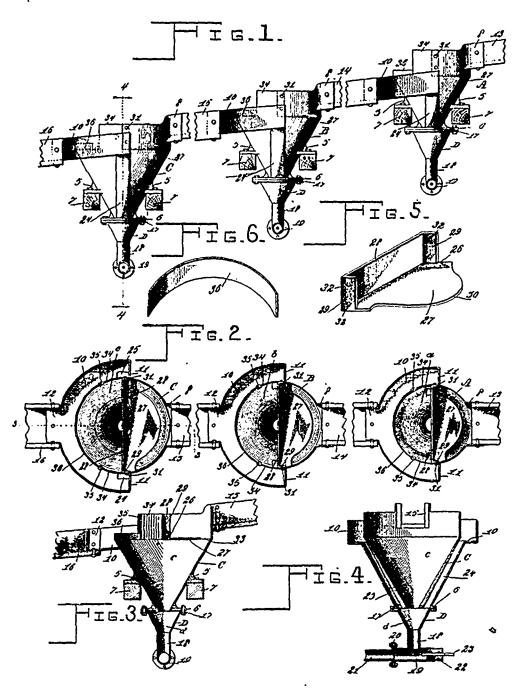
Culver Classifier-Used in Slocan Star Mill.
