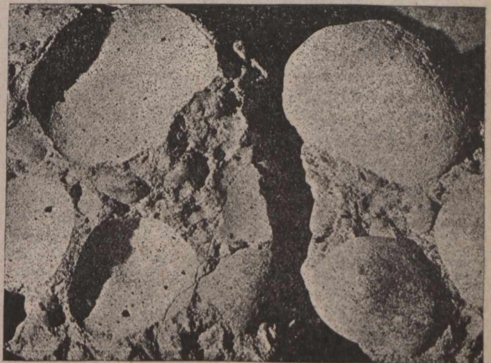
Fig. 8—Surface Contact Between Under Side of Gravel Particles and Mortar Bed, 1:2:4 Mix
