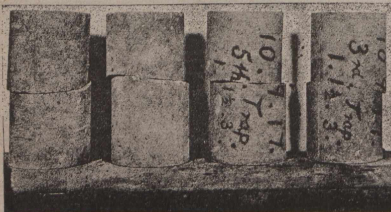
Fig. 4—Test Specimens: Consistency-Abrasion Test
