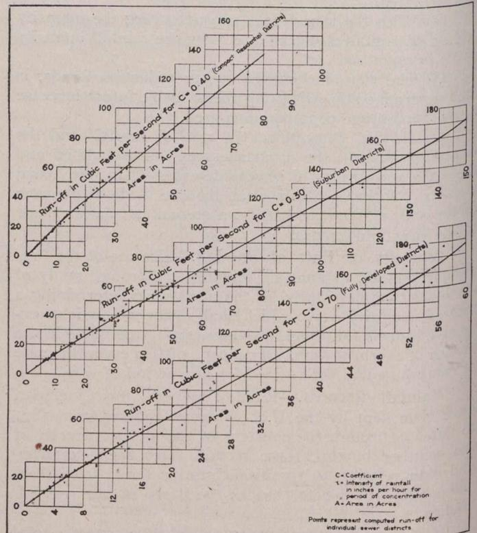
**Fig. 3.—Storm Water Run-Off, by "Rational Formula"**
