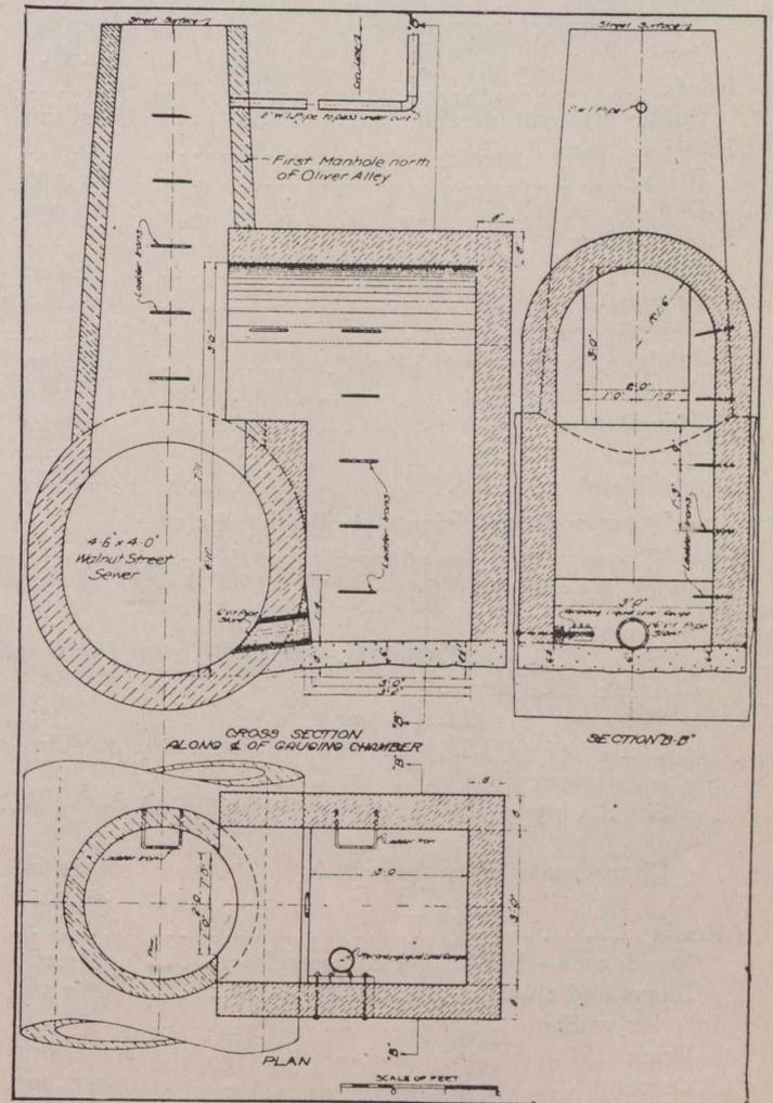
Fig. 4.—Details of Typical Gauging Chamber.
