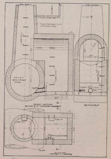
Fig. 4.—Details of Typical Gauging Chamber.
