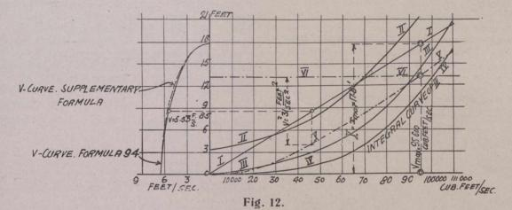
$$v^{2} = v_{2}^{2} - \frac{e}{B^{2}} \int_{0}^{x} x e^{D} dx$$
