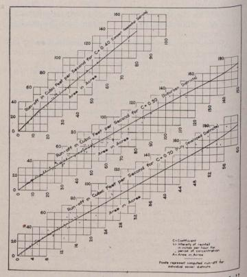
Fig. 3.—Storm Water Run-Off, by "Rational Formula" Q = A C i
