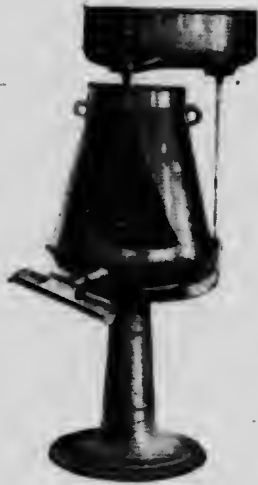
CIRCULAR MILK COOLER WITH COVER TO PROTECT MILK FROM AIR WHILE COOLING.
