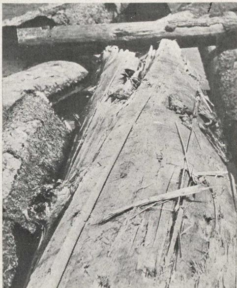
This is what is called a "spiral grain" spruce log. Because the tree grew with this defect, all such logs were discarded for aeroplane manufacture and indeed for nearly any other timber purpose.
