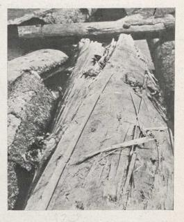
This is what is called a "spiral grain" spruce log. Because the tree grew with this defect, all such logs were discarded for aeroplane manufacture and indeed for nearly any other timber purpore.
