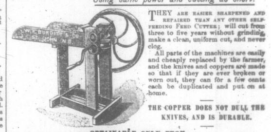
THEY ARE EASIER SHARPENED AND REPAIRED THAN ANY OTHER SELF-FEEDING FEED CUTTER; will cut from three to five years without grinding, make a clean, uniform cut, and never clog. All parts of the machines are easily and cheaply replaced by the farmer, and the knives and coppers are made so that if they are ever broken or worn out, they can for a few cents each be duplicated and put on at home.
