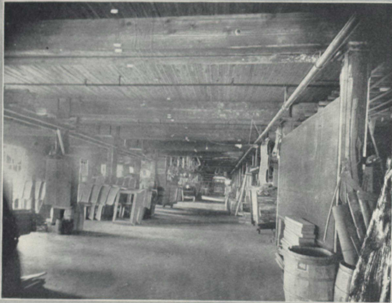
BODY ROOM OF THE McLAUGHLIN CARRIAGE COMPANY As far as the eye can see in the picture there are cutter bodies ready for the trimmers
